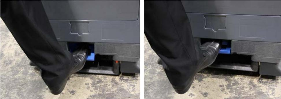
To change from Dolly to pallet, apply a **FULL** pressure on the pedal. This ejects the bearers and your Pally is now on pallet form.
